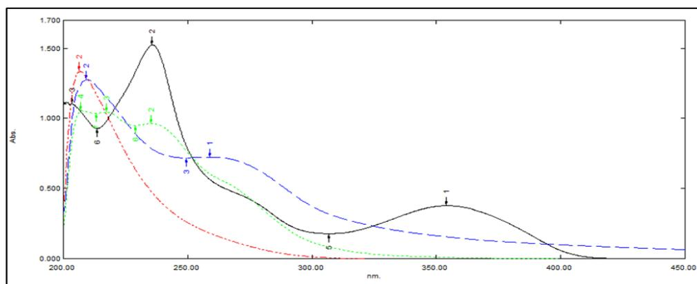
Figure 1. Zero order spectra of nimodipine 10 µg mL<sup>-1</sup> (\_\_\_\_) and 10 µg mL<sup>-1</sup> of its alkaline degradate (\_\_\_\_), 10 µg mL<sup>-1</sup> of its acidic degradate (....) and 10 µg mL<sup>-1</sup> of its oxidative degradate (-.-.-).
