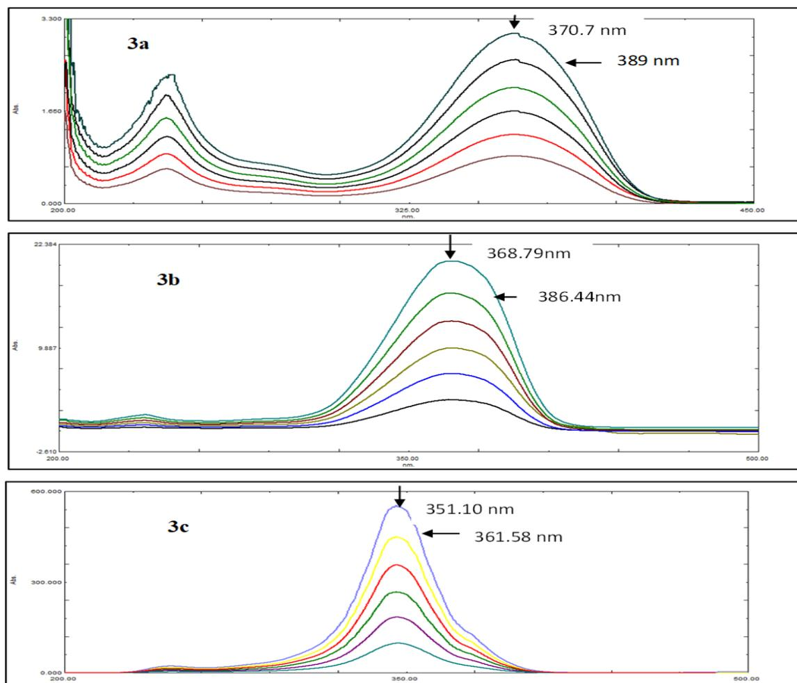
**Figure 3.** Ratio spectra of ( $3\text{-}18\ \mu\text{g mL}^{-1}$ ) of nimodipine using: a), ( $9\ \mu\text{g mL}^{-1}$ ) of its alkaline degradate as a divisor, b) ( $6\ \mu\text{g mL}^{-1}$ ) of its acidic degradate as a divisor, c) ( $10\ \mu\text{g mL}^{-1}$ ) of its oxidative degradate as a divisor.
